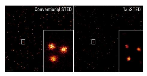
STED and DNA origami imaging: TauSTED 775 delivers resolutions <30nm on GATTA-Bead R whose nominal size is 23 nm. Scale bar: 1 µm.
